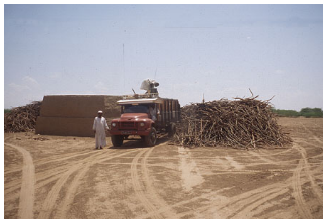
Figure 2: This picture, taken in 1996, shows the significant amounts of fuelwood required to fire a traditional clamp kiln. Transportation costs are also high and have a significant impact on the environment. Photo: Practical Action / Mohammed Majzoub.
